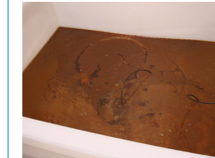
15 hours into the test. Exposed steel + electricity + water = lots of rust
