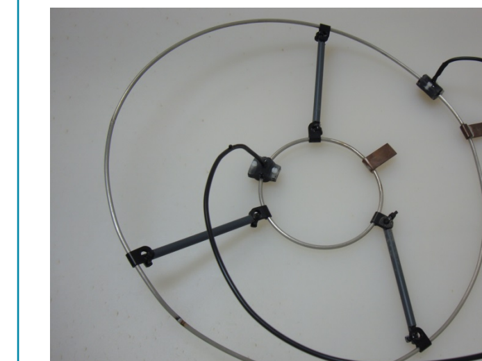
Stainless steel STREON rings prior to testing
