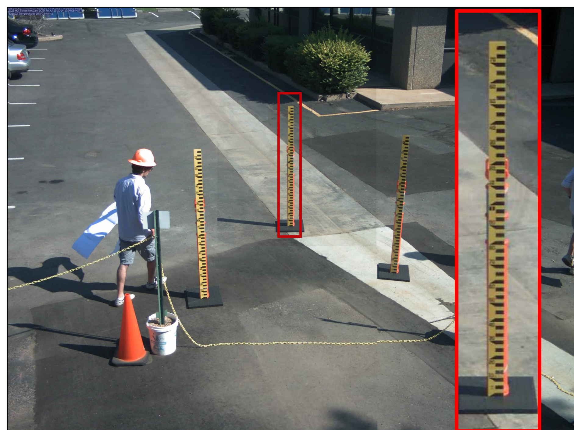
Figure 1. An example image of three staff gauges taken under the given setup parameters with a zoomed view of the region of interest outlined in red.
